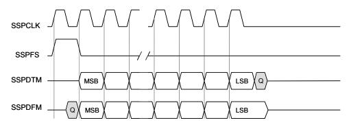
Figure 5.10-2 PCM Frame format for a single transfer
